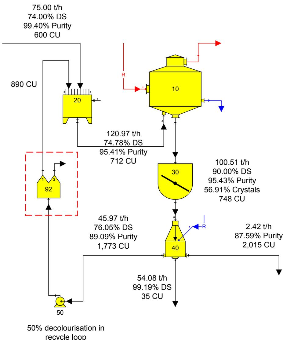
Figure 6 – Recycling single strike scheme with embedded decolourisation.
