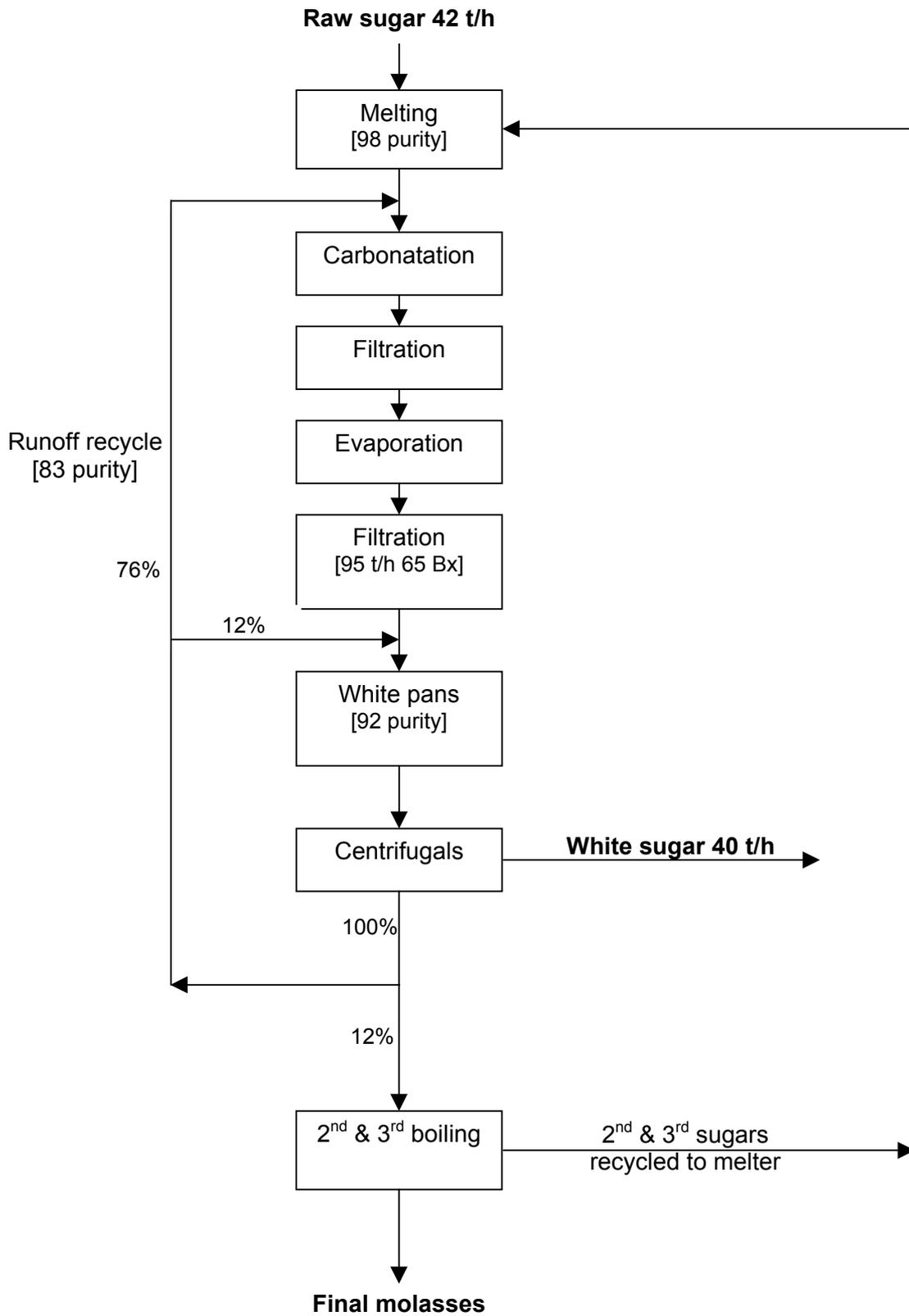
Figure 3 Simplified Flows in Russian Refinery Boiling Scheme
