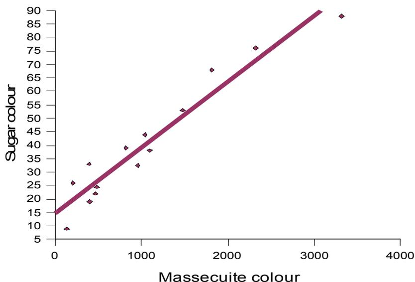
Fig 2. Collated Plant Data for R1-R4 Refined Sugar Strikes
